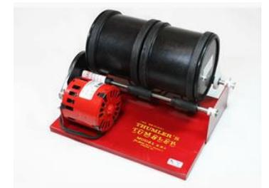
Fill tumbler barrels 1/2 to 2/3 full. Overfilling / underfilling yields poor results. We fill ours a little over 1/2 full.
